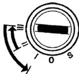
4. Turn key to the "III" to start. Release the key as soon as the engine has started, the key will automatically spring back to the "I" position.
