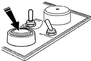
4. Press the starter button. Release the starter button as soon as the engine starts.
