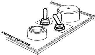
2. Activate the instrument panel by pressing the rocker switch downwards to "Power ON/OFF". The three warning lamps come on and can be tested.
