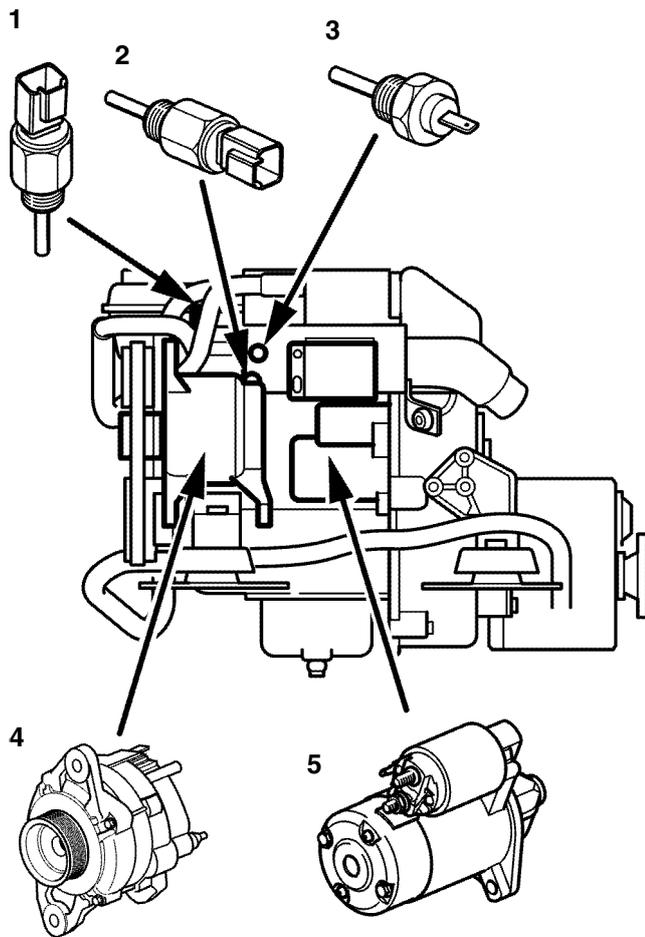
1. Engine coolant temperature switch D1-13, D1-20
